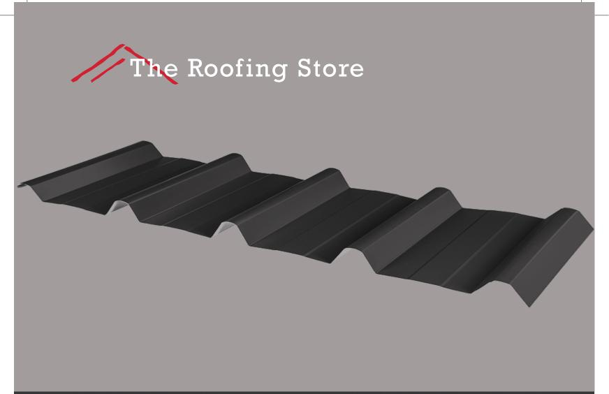
TRS 5 profile is designed for residential and commercial and wall cladding. It comes in G550 grade steel with minimum 0.40 mm BMT and maximum 0.55 mm BMT. The profile with 0.55 mm BMT gives greater resistance to high wind events such as tornado and cyclones.
