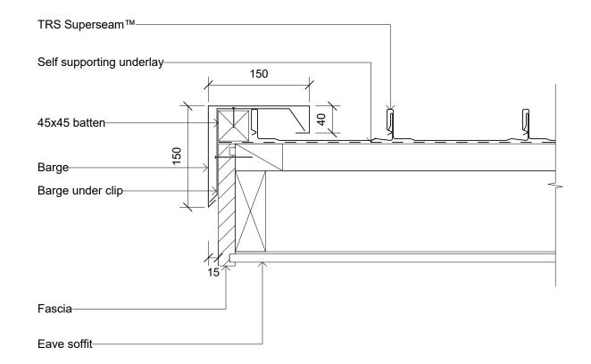
• These details are generally in accordance with E2/AS1 and or the NZ metal roof & wall caldding code of practice.
