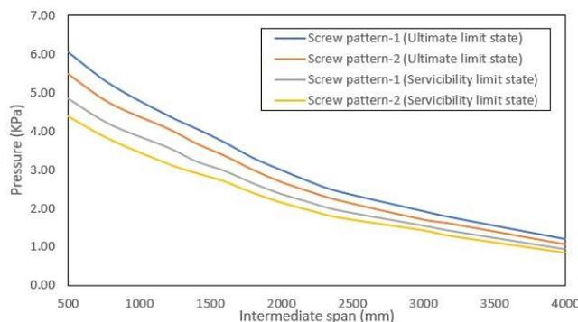
Wind load-span graphs for different types of screw patterns for 0.55 mm TRS 5 profile
