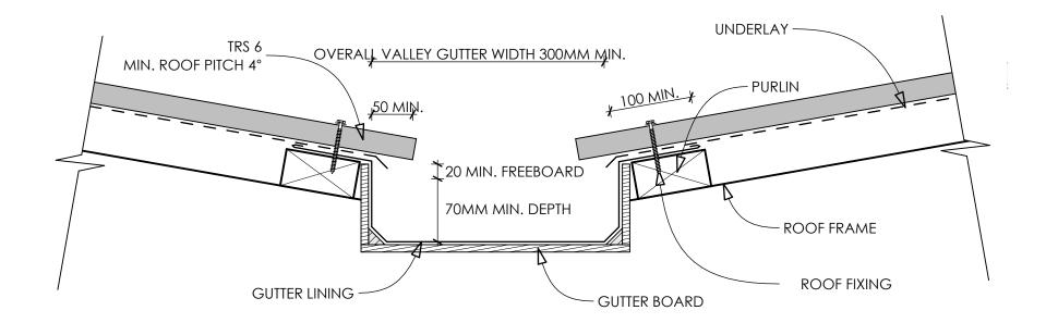
• These details are generally in accordance with E2/AS1 and or the NZ metal roof & wall caldding code of practice.
