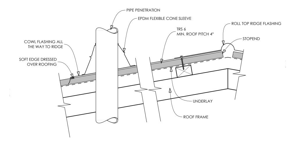
• These details are generally in accordance with E2/AS1 and or the NZ metal roof & wall caldding code of practice.
