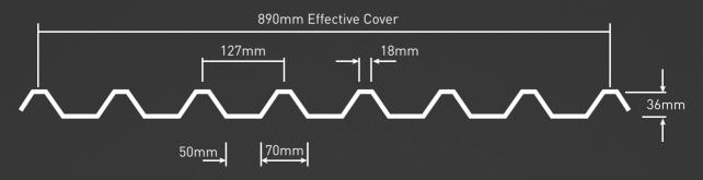
End SpanInternal SpanMinimum Pitch1.40m1.70m3°2.10m2.70m
