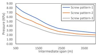
Wind load-span graphs for 0.55 mm BMT TRS Corrugated profile
