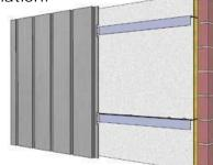
mechanical resistance (intrinsic weight and resistance to wind pressure), the maximum centre to centre distance between the brackets is 600 mm. The elbow brackets are fixed in place to provide cross fixing in the longitudinal direction of the panels.
