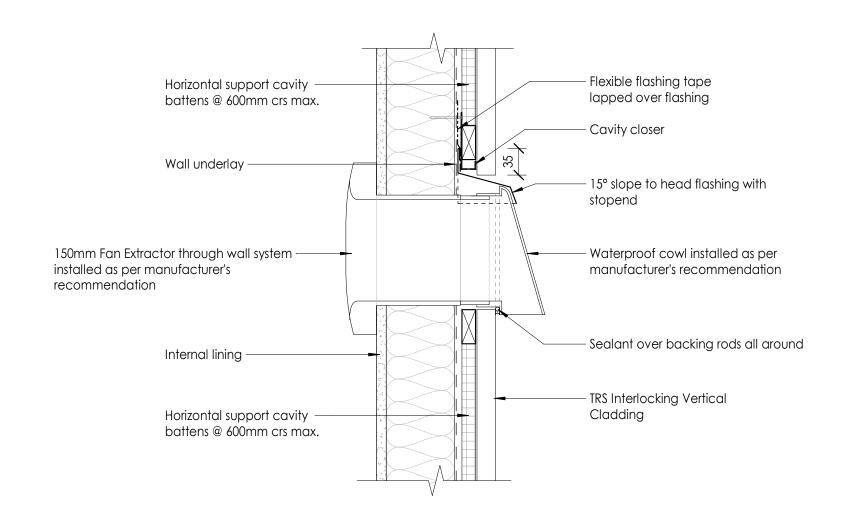
• These details are generally in accordance with NZBC E2/AS1 and or the NZ metal roof & wall caldding code of practice.
